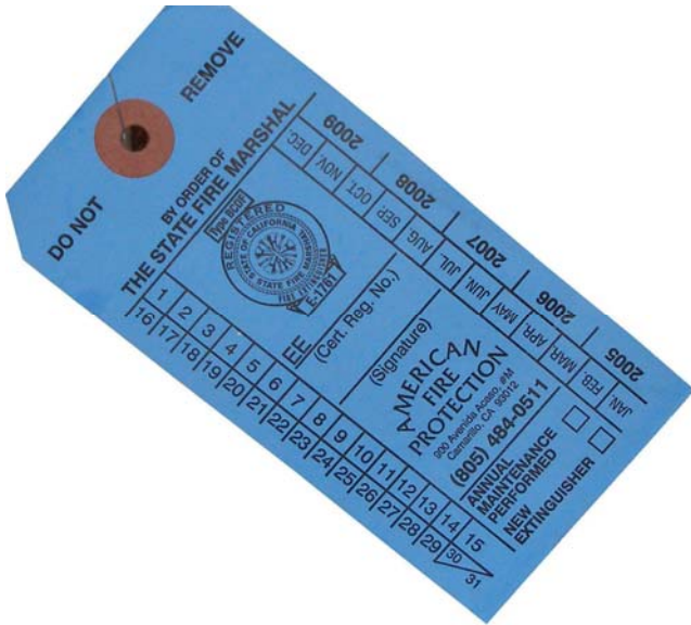
Inspection Tags Used by American Fire Protection
